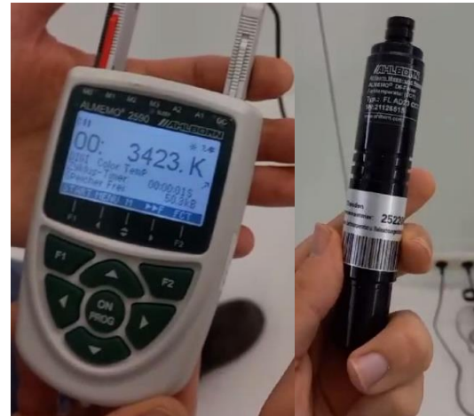
Figure 5: Color temperature sensor with device ALMEMO 2590-2.
